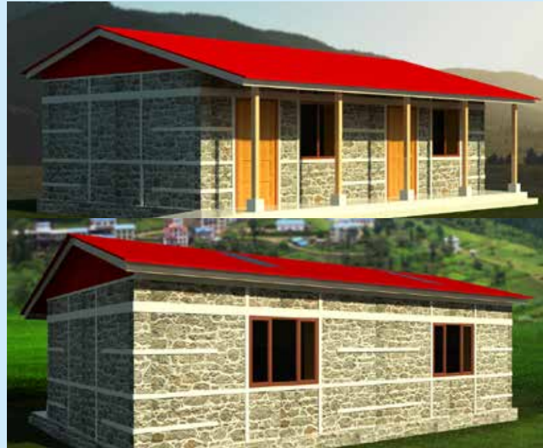
PHOTOS ABOVE: The proposed designs for the new school buildings feature lightweight timber-truss roofs supported on reinforced stone-masonry walls with reinforced-concrete horizontal bands.
